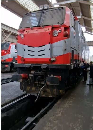
Figure 1 Wabtec ES30 Aci under preparations for retrofitting at ENR
